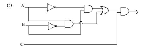
Allow [2 marks] for the NOT and AND gates applied to A and B, [1 mark] for correctly combining with an OR gate and [1 mark] for the final AND with C. [4 marks]
